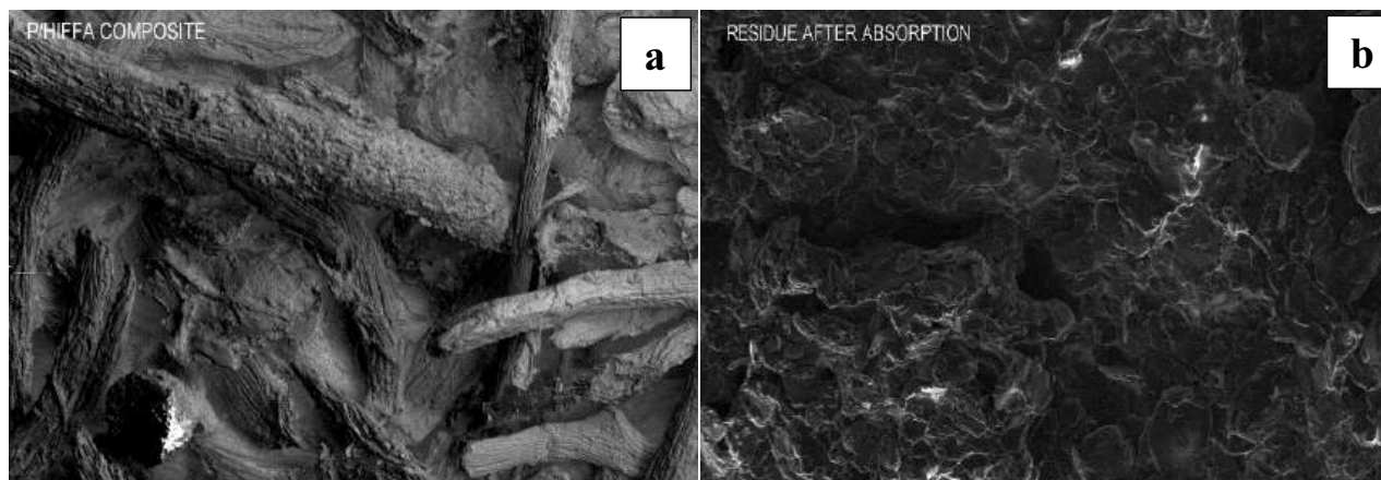
Fig. 3: SEM result for the PLCC (a)Residue after adsorption (b).
